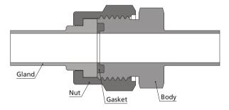
2. Tighten the nut 1/8 turn with a wrench while holding the fitting body steady.
