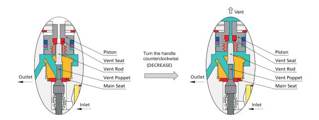
**RPGC Series Self-Venting Mechanism Diagram (Media Shown in Cyan)** Note: View the corresponding animated illustration on FITOK's official website.
