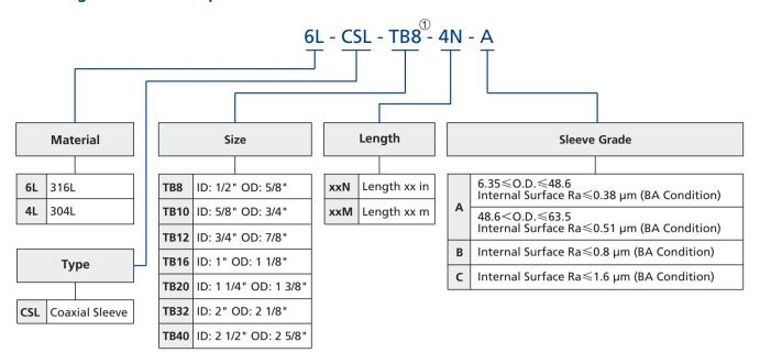
① Refer to outer tube outside diameter for sleeve part number selection.
