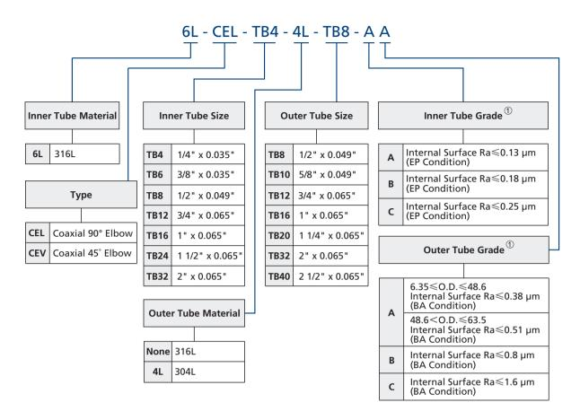
① Ra values for the internal and external surfaces of the cold working area of the fittings are not defined.
