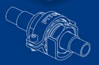
Thread the cap screw through the large hole on the strap and into the threaded hole on the collar. Snug with 3 mm hex key.
