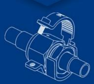
Insert the strap wing tab into the wing tab slot on the collar. Swing the strap to meet the collar.
